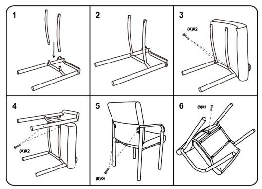
Insert and loosely tighten all screws. When assembly is completed, fully tighten all screws before using. This chair is only intended for sitting. Any other use will void the warranty.
